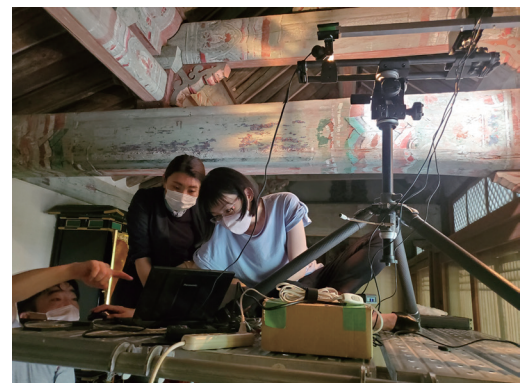
An on-site analysis of building coloring materials using portable analysis equipment (Tokyo National Research Institute for Cultural Properties)
