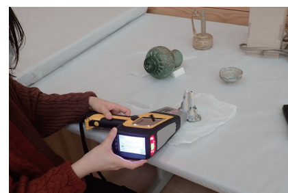
Determining the composition of a glass object owned by the museum with a handheld X-ray fluorescence spectrometer. (Kyushu National Museum)
