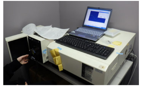
Spectrophotometric measurement of exposed dyed silk cloths (Tokyo National Research Institute for Cultural Properties)
