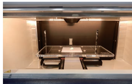
X-ray fluorescence analysis of corroded metal samples (Tokyo National Research Institute for Cultural Properties)
