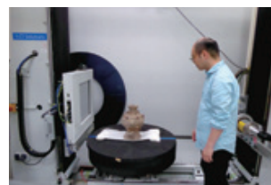
Surveying the structure of artifacts using X-ray computed tomography (CT) techniques
