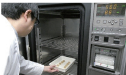
Testing insecticidal effect of humidity-controlled warm air treatment by studying the viable temperature for test insects (Tokyo National Research Institute for Cultural Properties)
