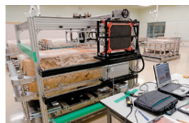
Investigation of the plaster layer of the Takamatsuzuka mural paintings using terahertz imaging technique
