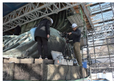
Survey by portable X-ray diffraction analyzer
