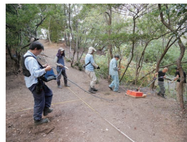
Survey using ground-penetrating radar (GPR) at the Itsukahara Kofun (burial tumulus) site (in Muko City, Kyoto Prefecture)
