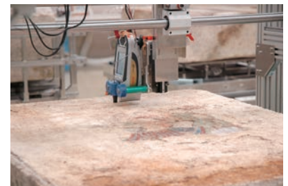
X-ray fluorescence analysis of mural paintings of the Takamatsuzuka Tumulus
