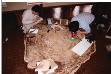
屋久杉円盤の年輪計測作業（森林総合研究所にて） Ring-width measuring of the Yakusugi disk at Forestry and Forest Products Research Institute
