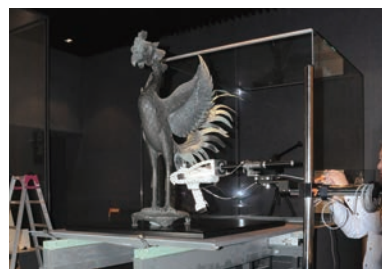
On-site analysis of a metal object by a handheld X-ray fluorescence spectrometer
