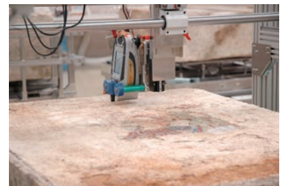
X-ray fluorescence analysis of mural paintings of the Takamatsuzuka Tumulus
