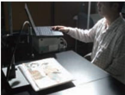
浮世絵彩色材料の可視反射分光分析 On-site analysis of color materials used in an ukiyo-e print by visible reflection spectroscopic method
