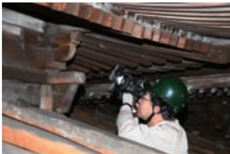
国宝永保寺開山堂の屋根葺替修理工事に伴う年輪年代調査 Dendrochronological research of the National Treasure: Kaisando Hall, Eihoji Temple in Gifu Prefecture as the roofing repair work
