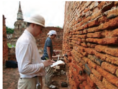
アユタヤ遺跡における煉瓦の含水率測定 Measurement of water content of the bricks at Ayutthaya Site, Thailand
