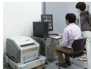
Investigation by X-ray radiography using a portable scanner
